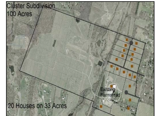
Above (top to bottom): Example of a conventional versus a conservation subdivision. The above illustrates how a conservation subdivision can be used to retain large tracts of farmland. The illustration above shows a conventional subdivision of 100 acres into 20 five-acre lots where the community’s Zoning requires a minimum lot size of five acres per lot. The illustration below shows a conservation subdivision where the 20 building lots are clustered on 33 acres of the site – leaving 67 acres of prime farmland within a conservation easement. The conservation easement can be held by a homeowners association, land trust, or sold to an adjacent farmer for the agricultural value of the property that is far lower than the use value if it could be developed. 89
